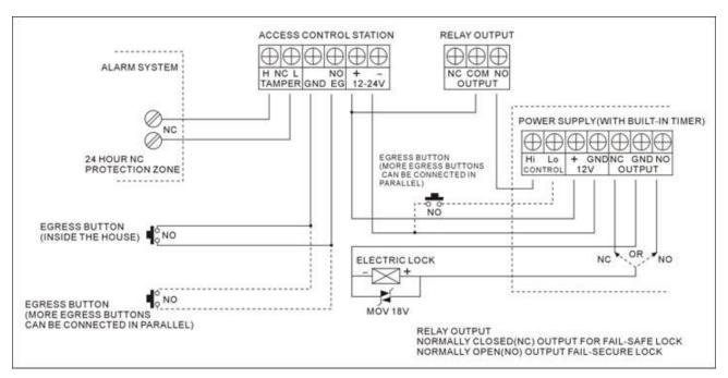
(2)The Control Station directly controls the connecting apparatus (Note: Max Rating of Relay Contact Current 3A / 24VDC)
